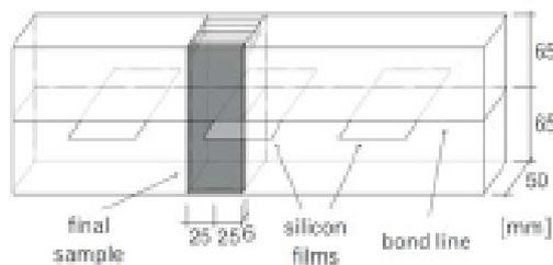
Figure 5: Sample preparation and geometry
