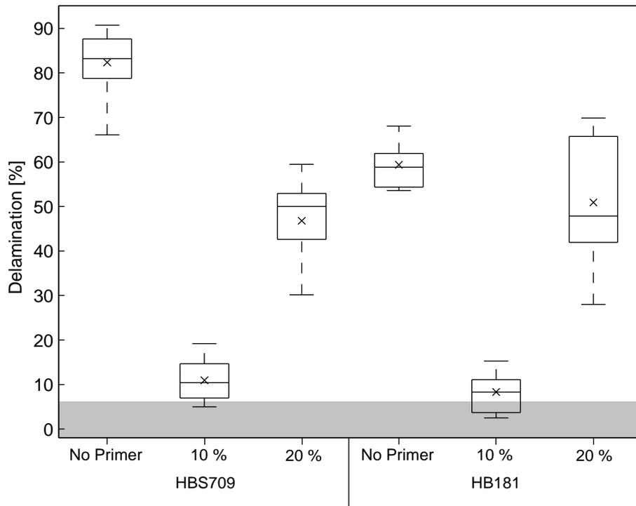
Figure 12: Delamination results for ash wood and priming with different 1 C PUR and priming with no Primer, 10 % and 20 % primer concentration for the adhesive HBS709 and HB181, serie 2
