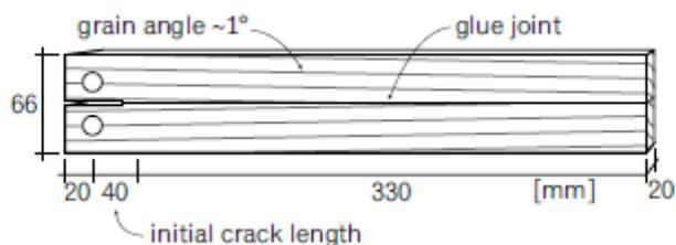
Figure 7: DCB geometry, in [mm]
