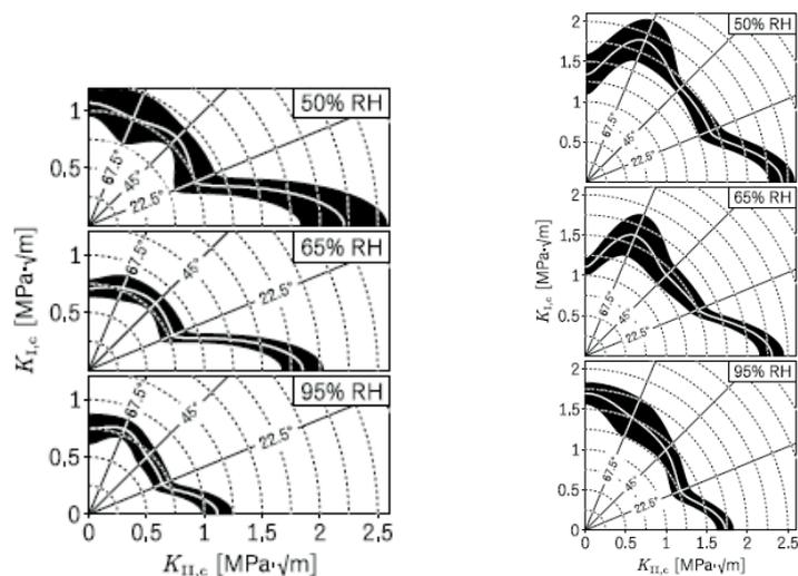
Figure 8: Fracture toughness'  $K_{c}$  for 1 C PUR (left) PRF (right) and different RH with CI (confidence interval) in black area)
