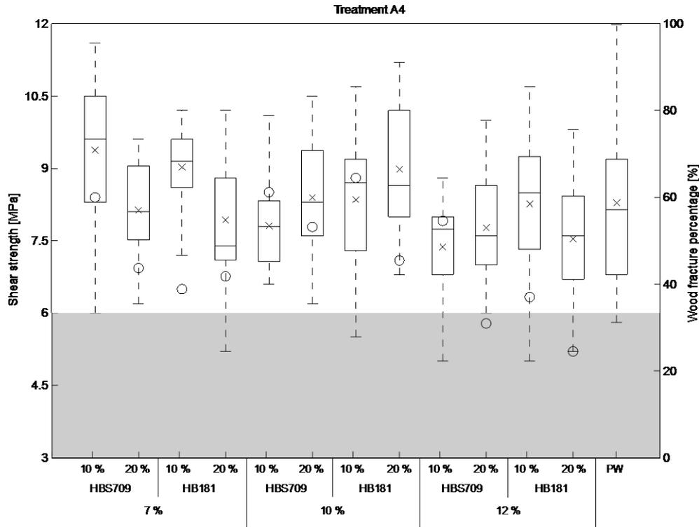
Figure 10: Tensile shear strength and wood fracture percentage after treatment A4 for ash wood and different adhesives for gluing with different moisture content, adhesives and primer concentration (pw = plain wood samples)
