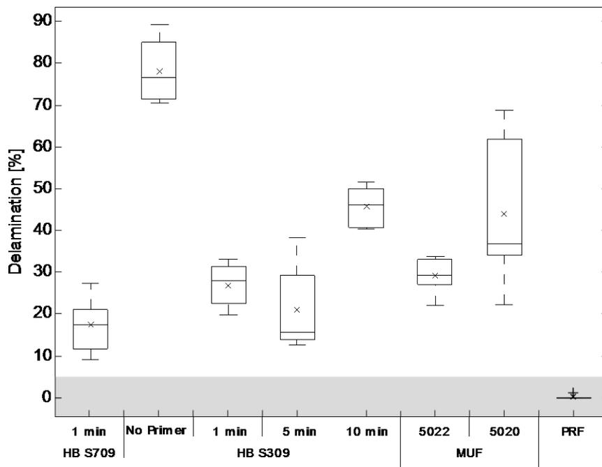
Figure 11: Influence of the Primer Influence Time (PIT) of 1C-PUR on the delamination during the preliminaries experiment in comparison with MUF (Preferre 4546/5020 and Preferre 4546/5022) and PRF (Aerodux 185) system – delamination test according to the high temperature cycle (DIN EN 302-1:2013), serie1
