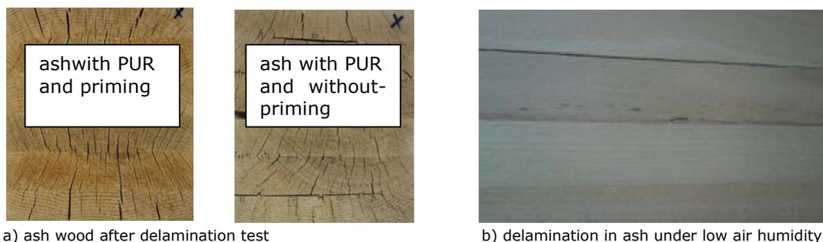
a) ash wood after delamination test
