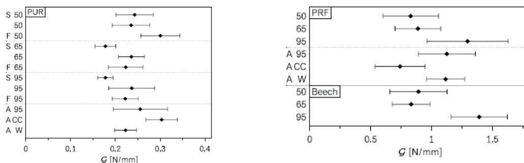
Figure 9: Fracture energy for glued wood PUR and PRF and for beech solid wood
