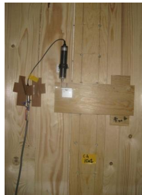
Figure 10: Relative slip in plane wall-to wall connection
